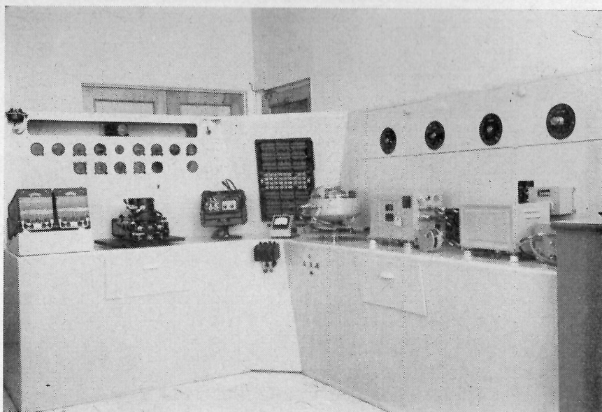
BRITANNIA TEST STAND. Set up for checking instrument system of Canadian Pacific Air Lines' Britannias, this test stand is part of the facilities of S. Smith and Sons (Canada) Ltd. Company also has dustproof instrument lab at Don Mills, Ont., plant.
