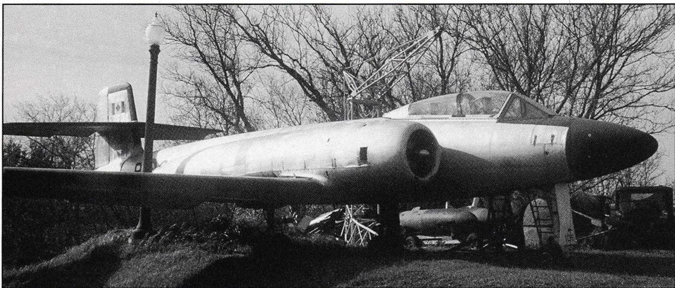
One of the oldest CF-100s in Canada 18106. It is easily identified by its smaller streamlined nose.
