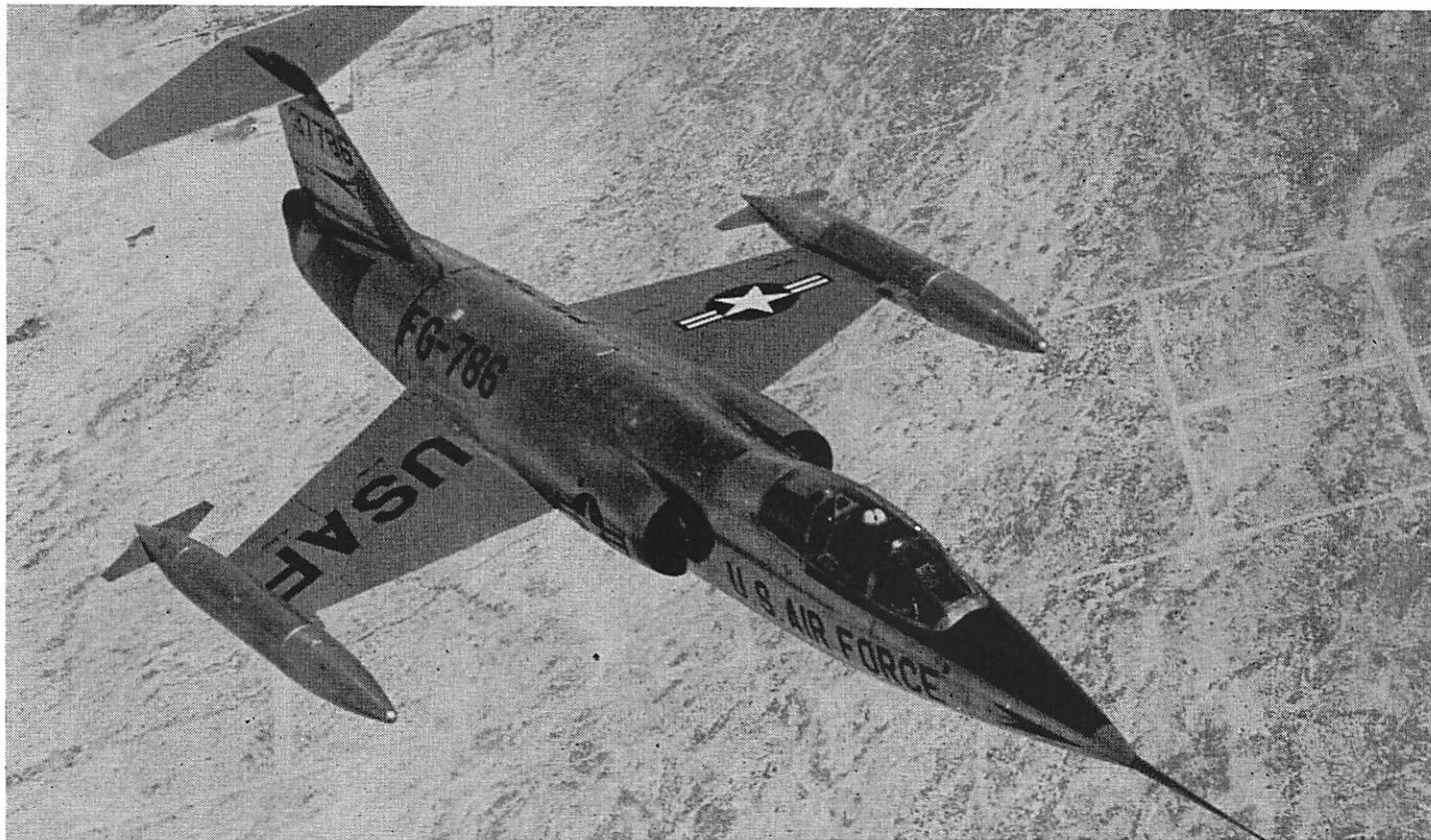
LOCKHEED F-104A STARFIRE new USAF supersonic night-and-day fighter powered by the General Electric J-79 engine with afterburner which develops half of its thrust as a ramjet. (Prototype powered with the Curtiss-Wright J-65 with afterburner, first flown, February, 1954). Now in quantity production it features: "most powerful jet engine, thrust per pound developed; first downward ejection" system for a production jet fighter; an all flying tail. Note unusual supersonic speed wing configuration. Wings are razor thin and so leading edge sharp protectors have to be put on on the ground.
