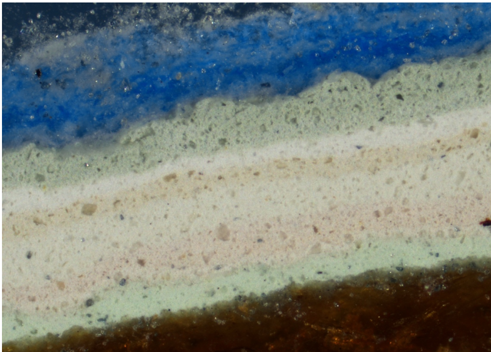
Figure 6 Photomicrograph of sample KH.W8 , removed from high on the west wall over the door. Note the roughly six layers of modern paint above previous wallpaper; the other seven wall samples were virtually identical. Bottom of sample and earliest wallpaper layers not shown. Visible light, 40x.
