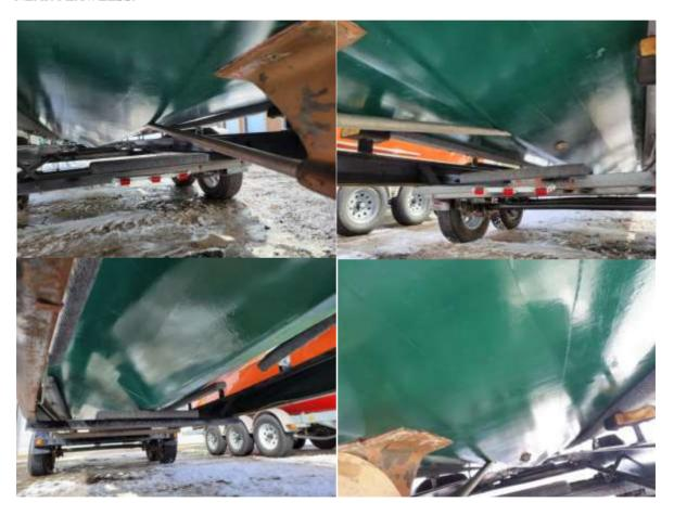
HULL PERCUSSION SOUNDINGS SHOWED CONTINUOUS STRUCTURAL INTEGRITY AND NO VOIDS, LOOSE SUB-STRAIGHT LAYERS OR HULL STRUCTURAL PROBLEMS WERE NOTED.
