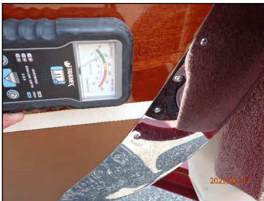
Obtaining Moisture Readings From Topsides
