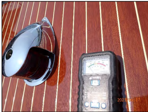
Obtaining Moisture Readings From Deck Surfaces
