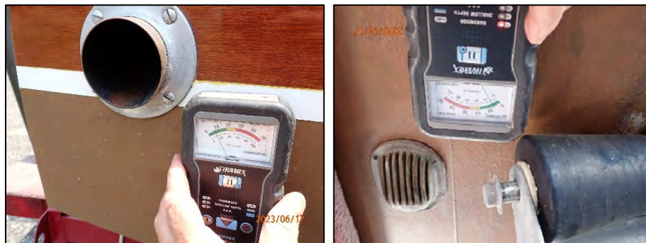
Obtaining Moisture Readings From Transom & Hull Undersides
