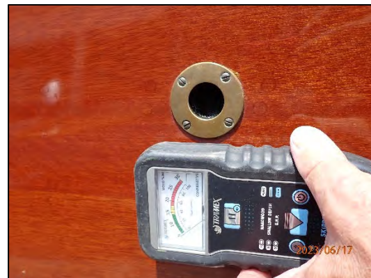
Obtaining Moisture Readings From Topsides
