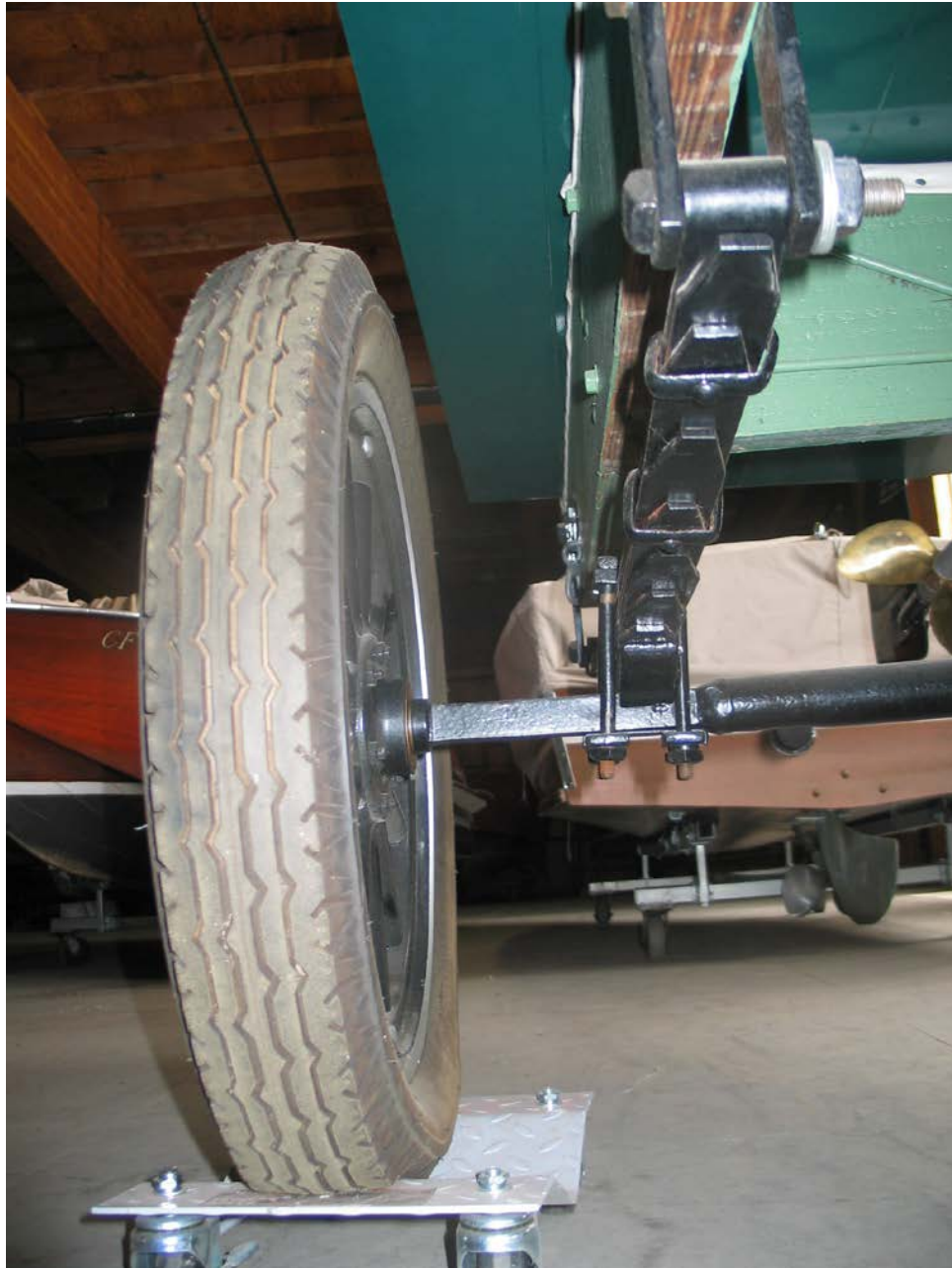
Restored Model-T wood frame period leaf springs hardware stored on dollies
