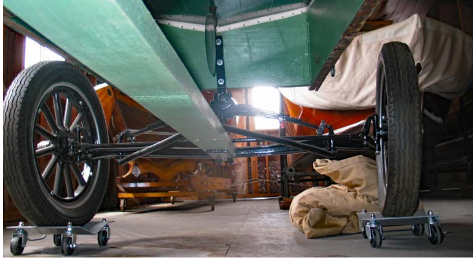
Rack & pinion carriage assembly intact appear serviceable
