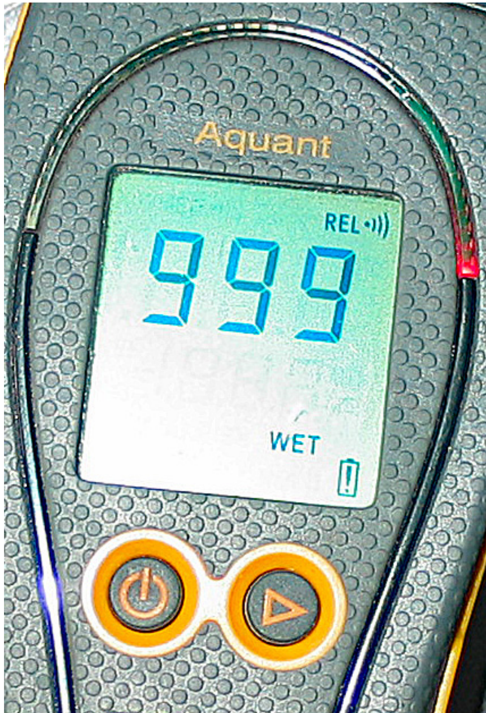
Protimeter Aquant meter bench mark recording high moisture content
