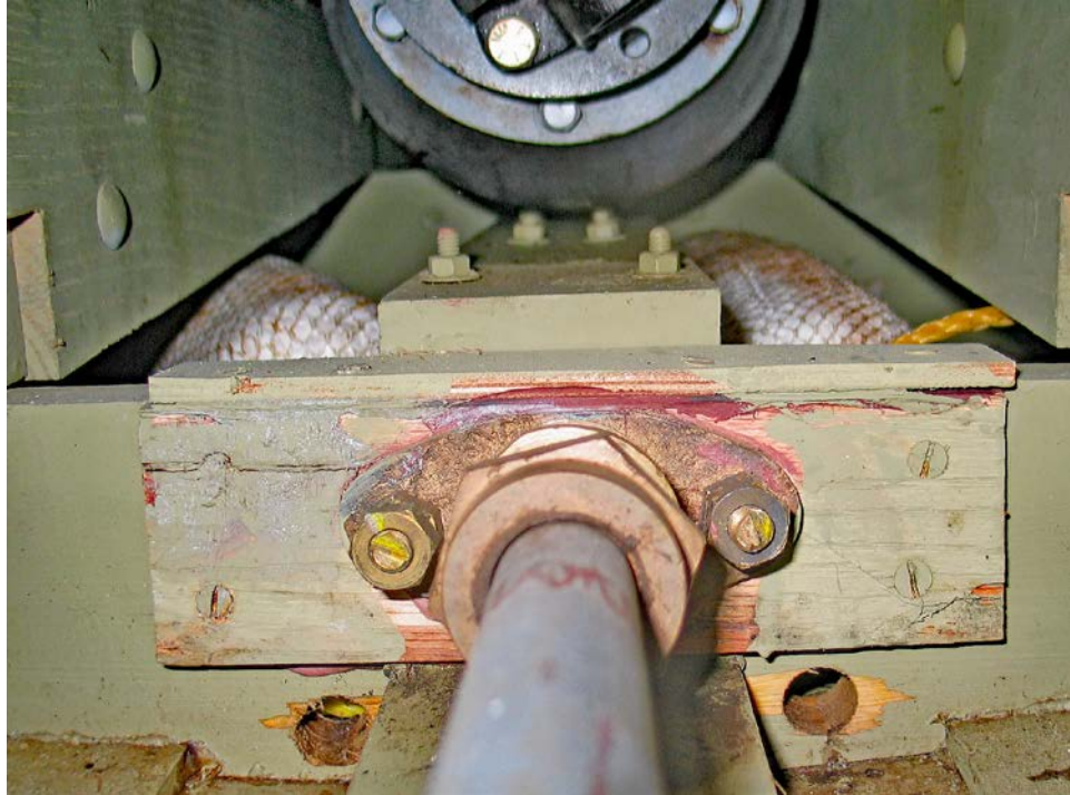
Shaft log, prop shaft, stuffing box inspected in a static condition appears serviceable
