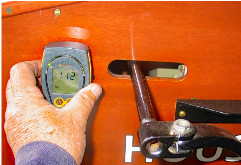
Protimeter Aquant meter recorded acceptable transom moisture content
