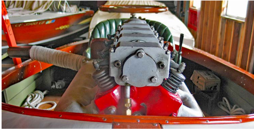
Peerless 151cid 4 cylinder overhead cam racing engine
