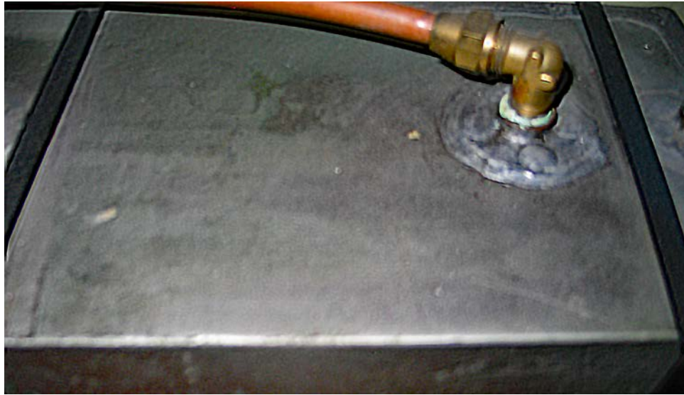
Upgraded aluminum fuel tank with copper fittings
