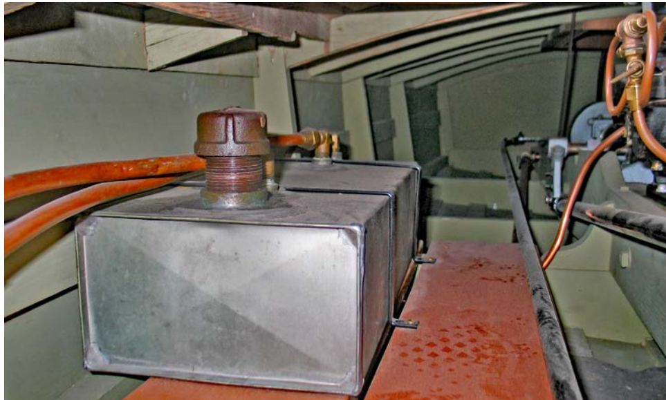
Upgraded aluminum fuel tank with copper fittings installed port amidships
