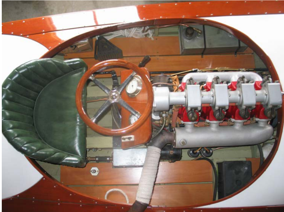
Winterized Peerless 151cid 4 cylinder overhead cam racing engine
