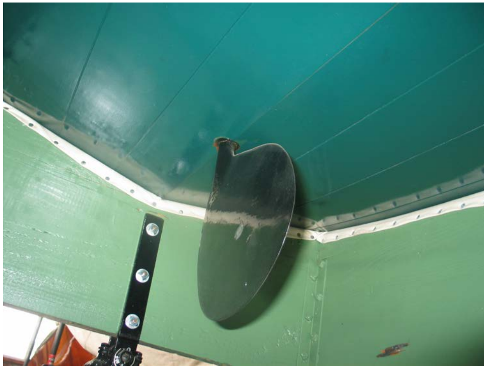
In addition to the transom spade rudder; the steering assembly includes a forward teardrop rudder
