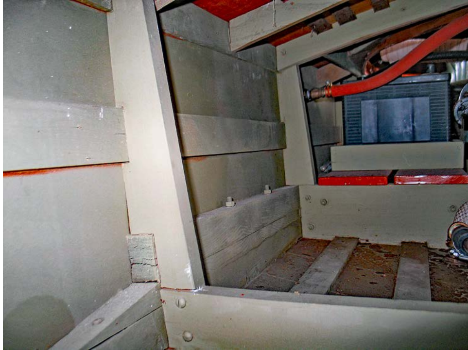
Plywood skin supported by battens & sawn frames; a few of the frames have dried & cracked
