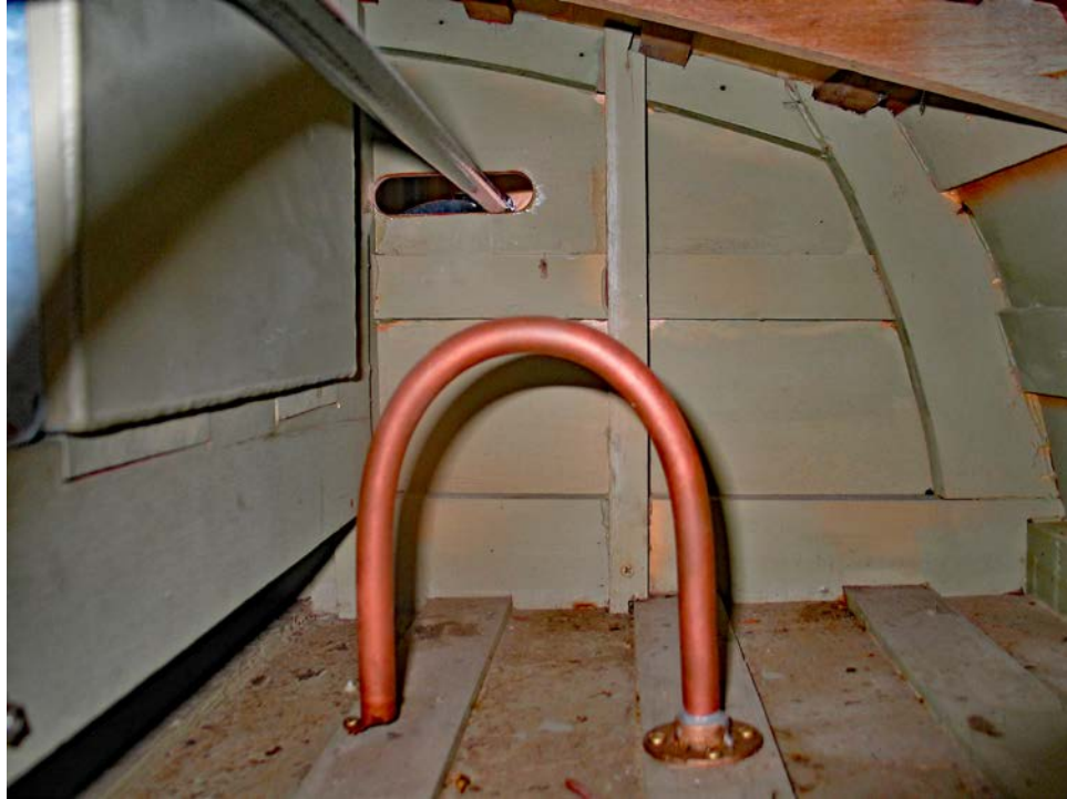
Syphon bailer installed port quarter
