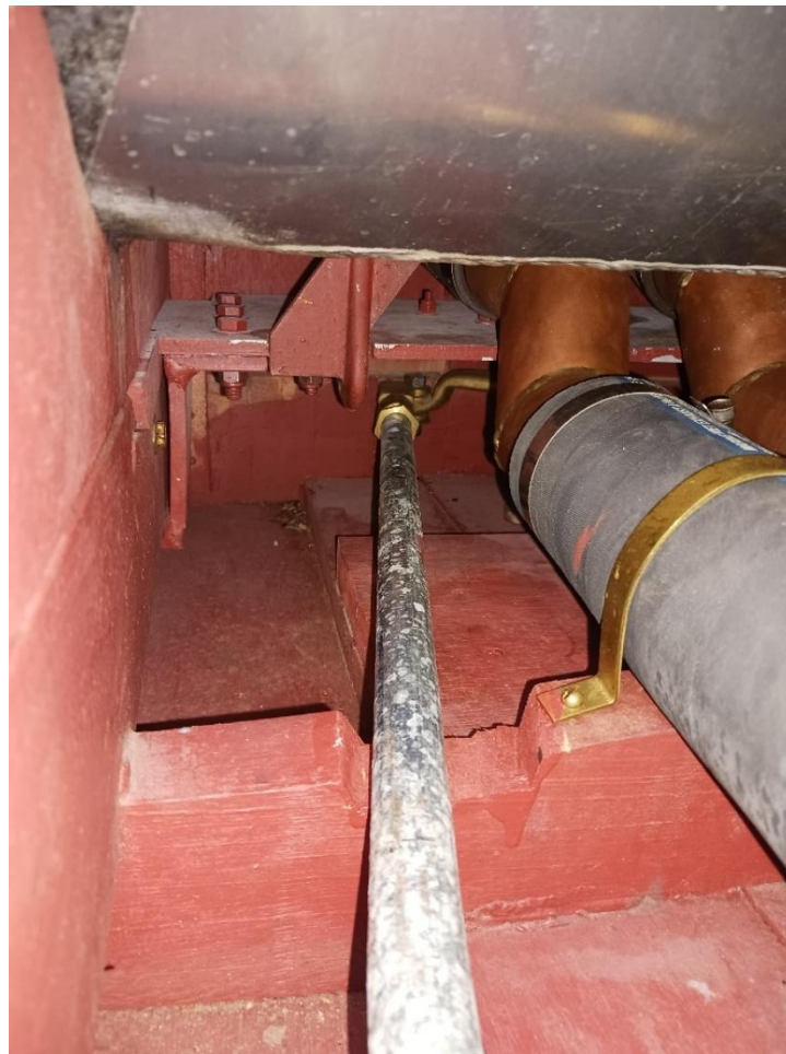
Exhaust are Trident Hose and Copper to transom
