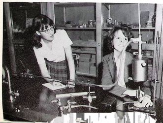
Seniors Ruth Baltrukenas and Mary Kalafus perform a physics experiment to determine the amount a metal rod expands when heated.
