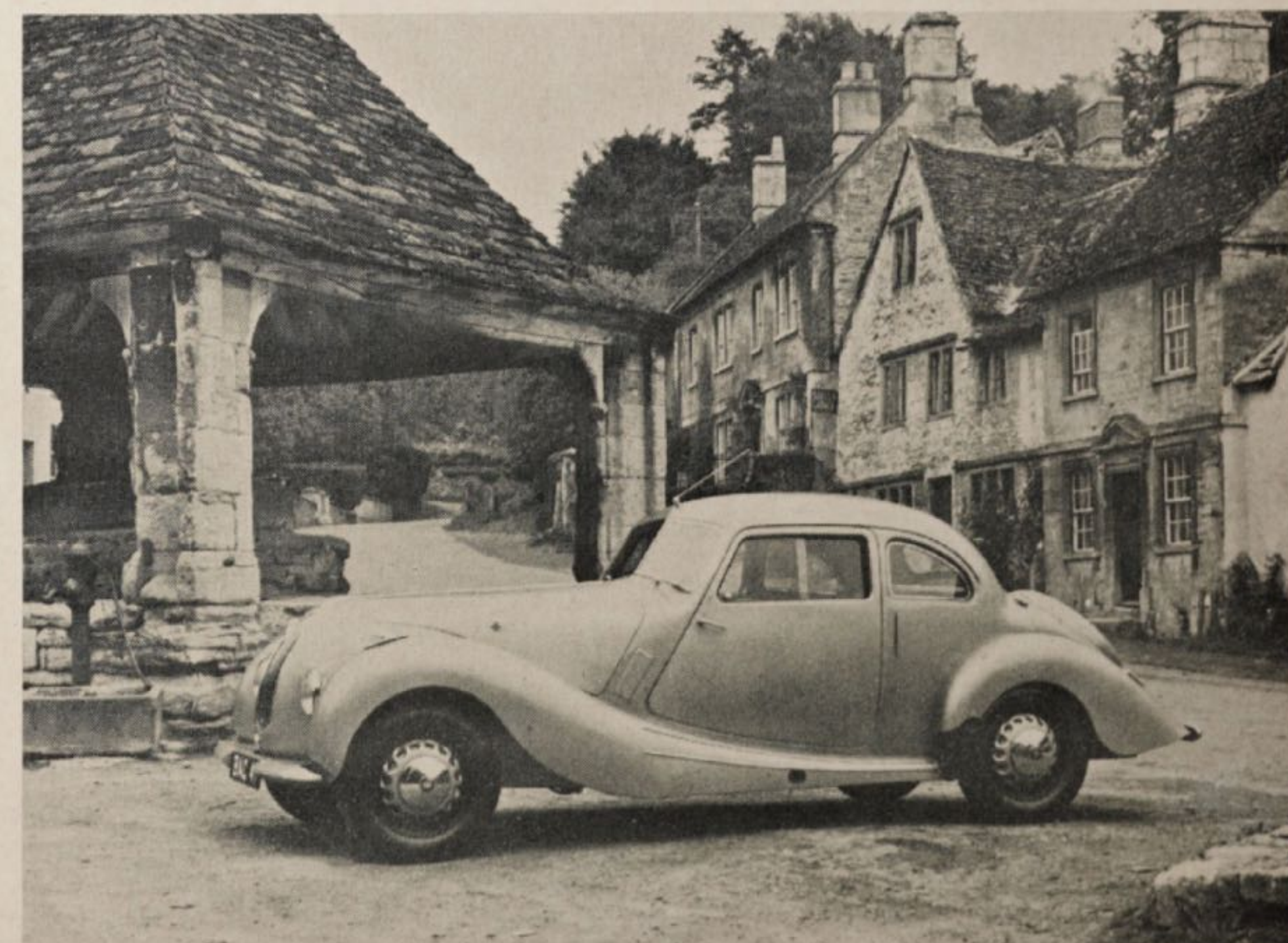
BRISTOL Type 400 saloon, with unitized frame construction, seats four and has wheelbase of 114 inches. Engine is six-cylinder of 1971 cc (122.2 cu. in.) capacity, producing 80 bhp at 4200 rpm. Aluminum head contains inclined ohv, pushrod operated. Suspension is by transverse leaf spring in front and torsion bars in rear
