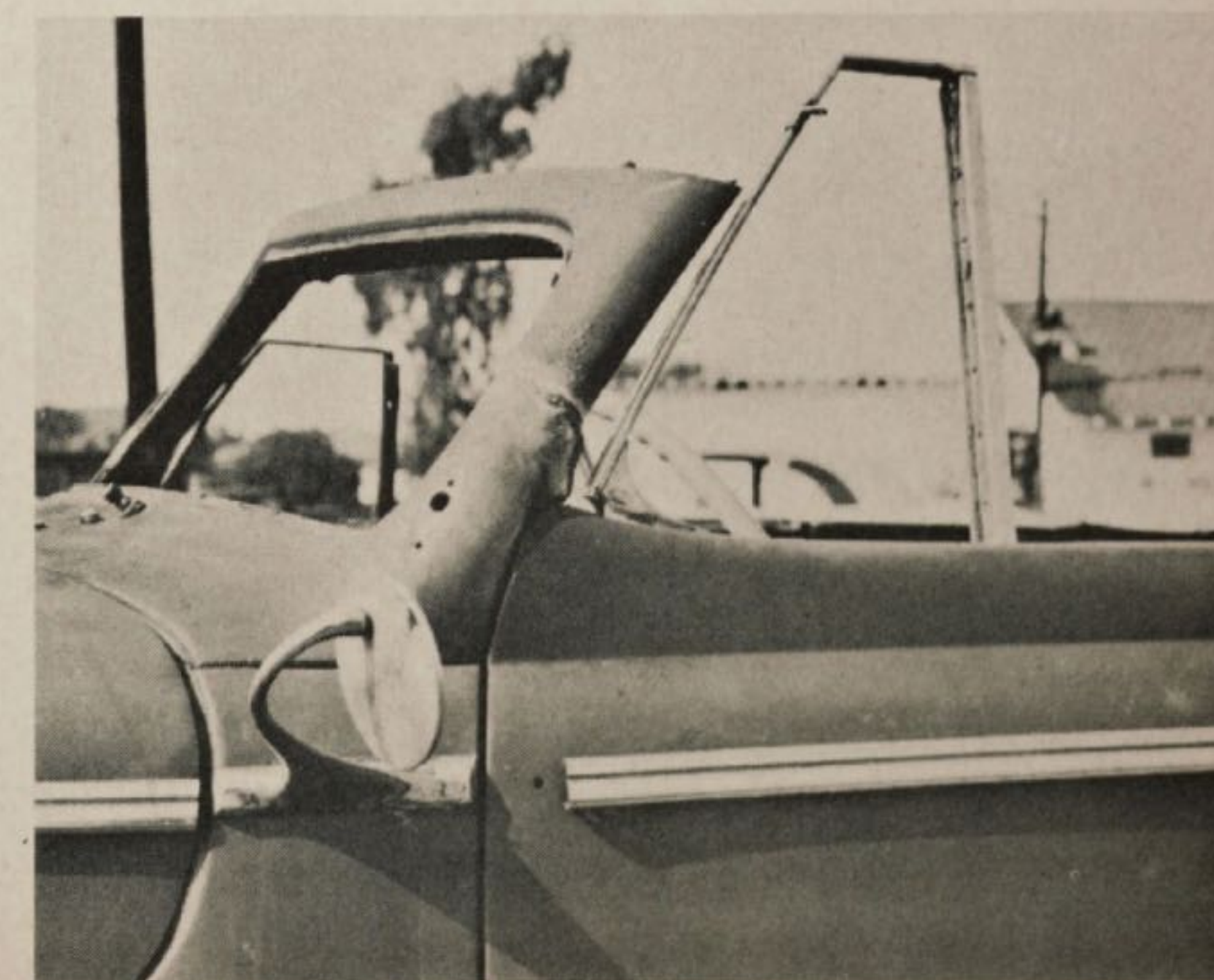
TOP of this '47 Merc has been chopped 5 1/2 inches. Note difference between top of windshield and top of quarter window
