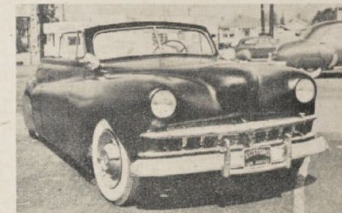
FINISHED product, a '41 Barris-Ford. Chopped, channeled, frame-and-body-sectioned, car has been completely sealed. Grille is both '49 Pontiac and '49 Stude
