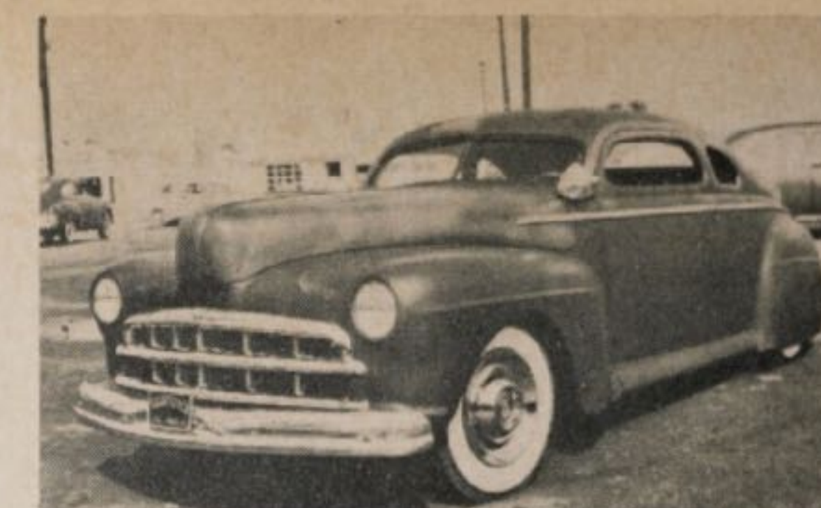
CUSTOMIZED '48 Merc coupe by Barris for Larry Robbins of Beverly Hills is ready for painting. Special underbase follows primer, then 8 gallons of color coat added
