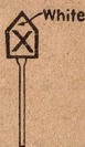
HIGHWAY GRADE CROSSING WHISTLE SIGN (1320 Feet from Crossing where Speed is 60 m. p. h. or less and 1850 feet where Speed is over 60 m. p. h.)
