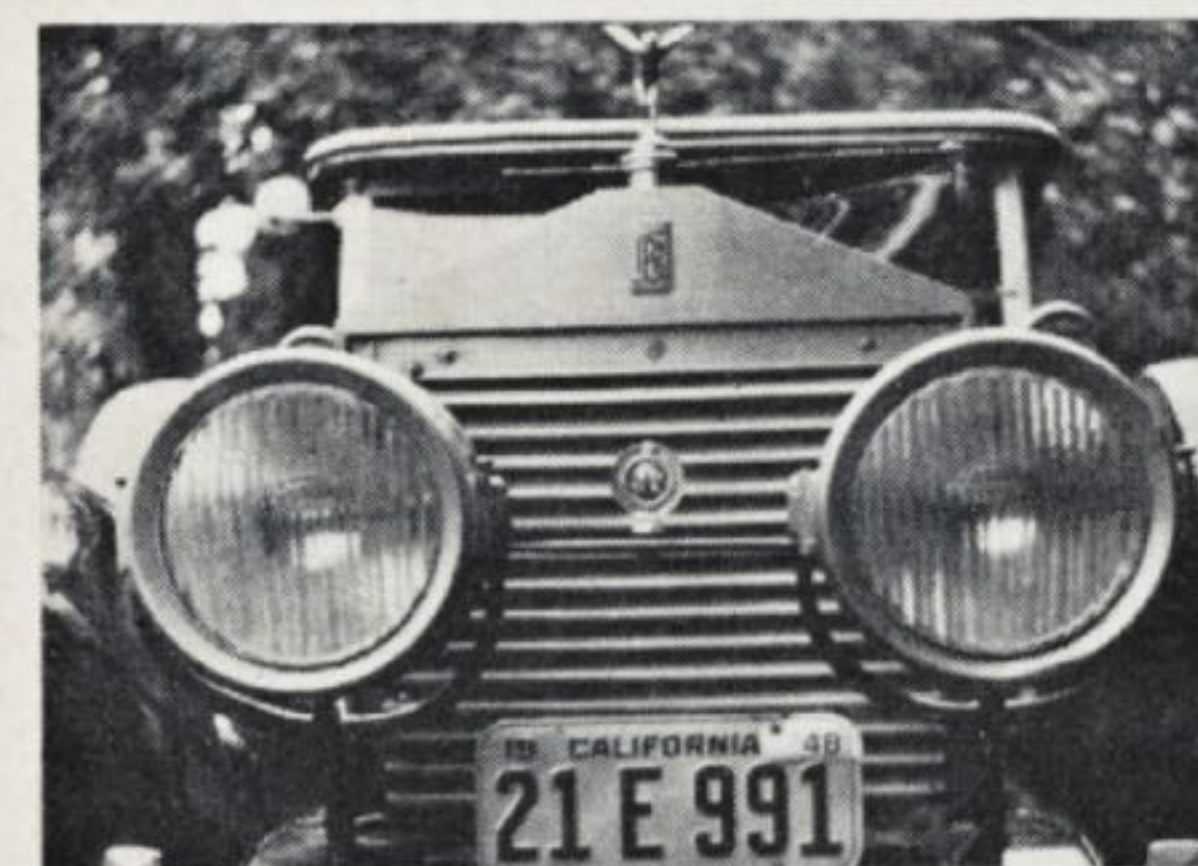
ROLLS-ROYCE Silver Ghost series can be identified by its horizontal radiator shutters. Shell is of solid nickel silver. Note huge headlights
