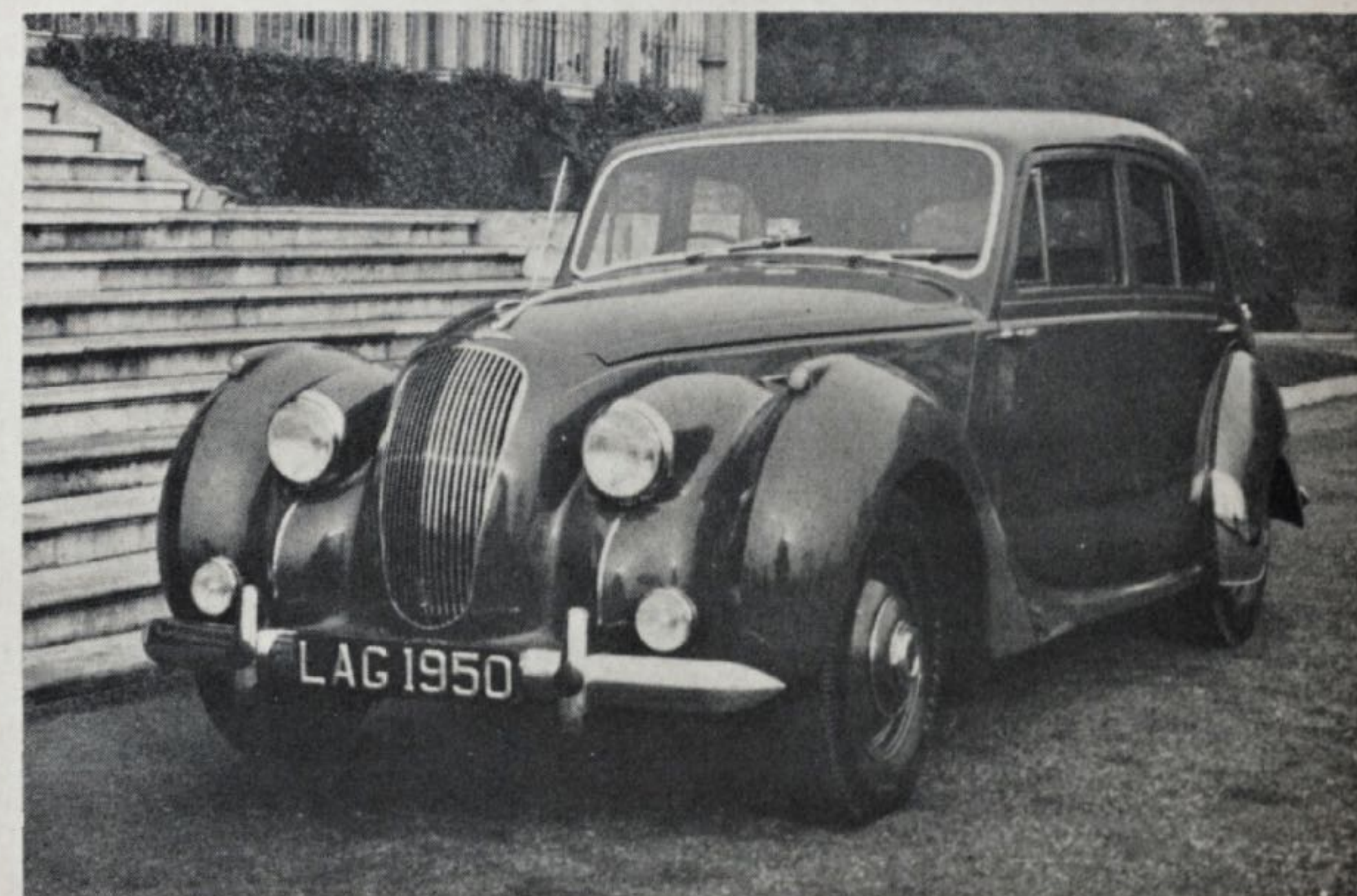
LAGONDA 2 1/2-litre sedan is entirely new throughout. With a six-cyl. engine of 163-cubic-inch capacity, power delivered is over 105 bhp at 5000 rpm. Compression ratio is 6.5:1. Like the Jaguar, twin overhead cams are used. The wheelbase is 113 1/2 inches, while the tread is 56 3/4 inches. An "X" frame is used, with independent suspension at all four wheels. Four speeds forward are provided, with a rear axle ratio of 4.56:1. Lagonda seats five or six passengers comfortably
