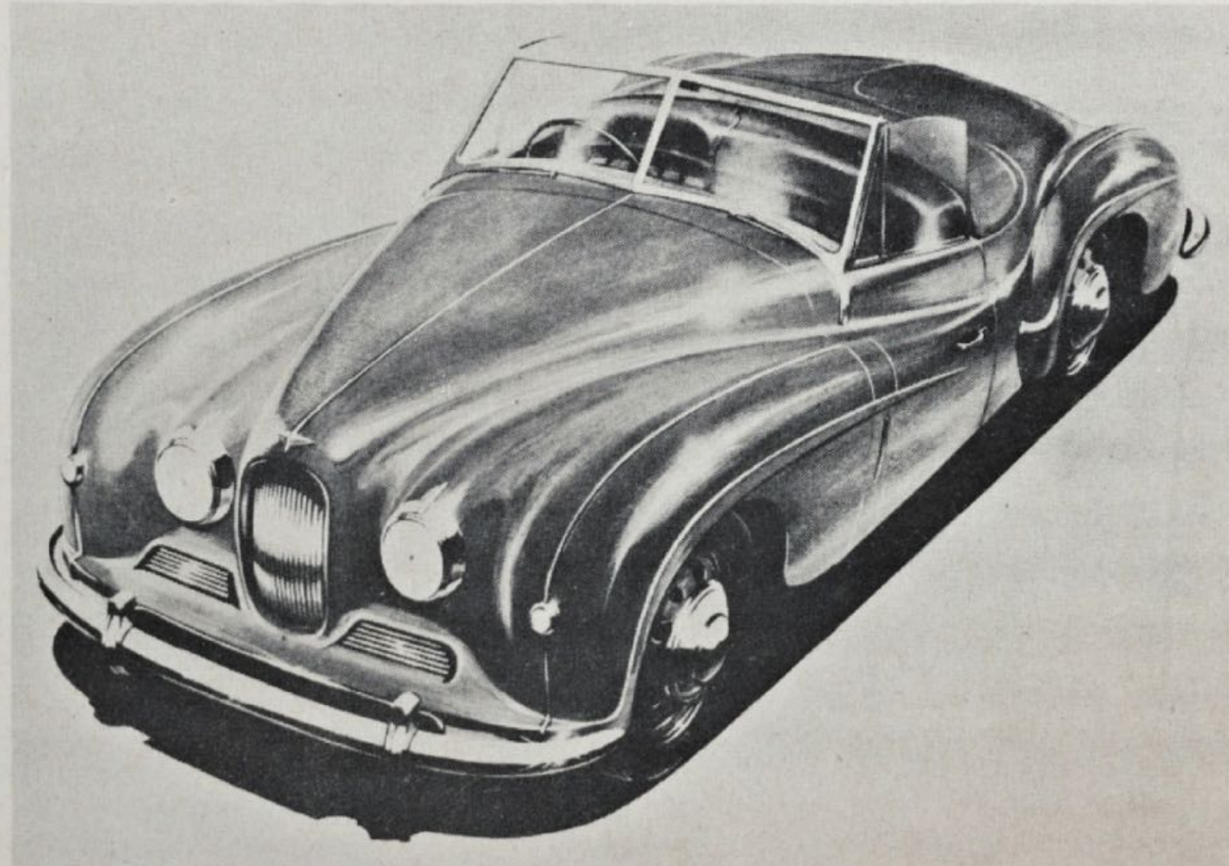
JOWETT Javelin Jupiter, newest of Britain's sports cars, which will be seen for the first time in the United States at the British Motor Show. The Jupiter is adapted for road racing as well as for regular use, with full convertible coupe equipment—sliding windows, a snug top, and top performance in low and high speed ranges. It seats three. Engine is four-cyl., horizontally-opposed, of 90.59 cu. in. displacement, delivering 60.5 bhp. Top speed is over 90 mph, acceleration good
