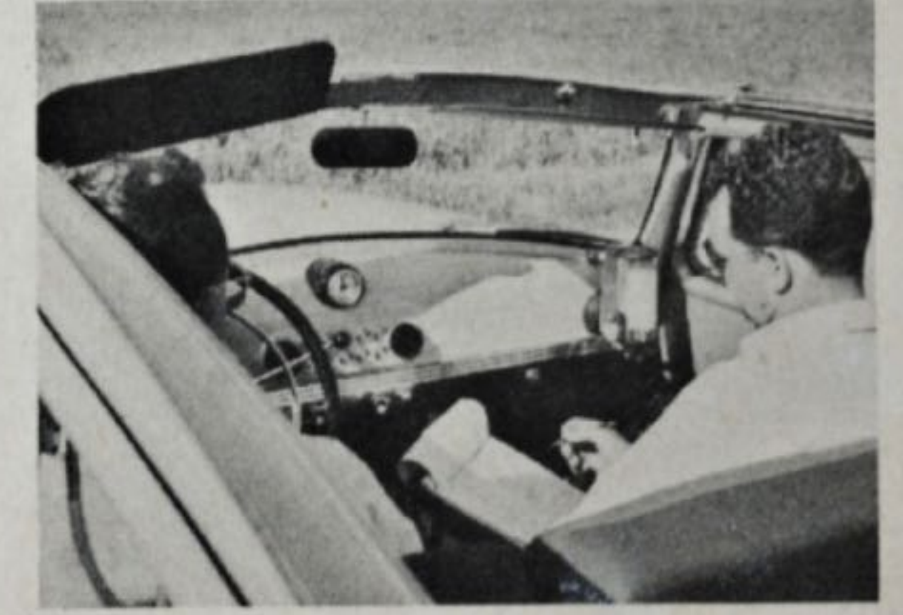
TECHNICAL Editor records mileage reading after one of the fuel consumption runs. Note fuel foaming up as it fills consumption meter
