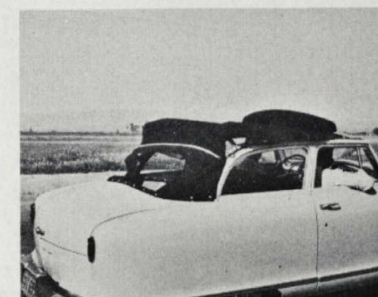
CONVERTIBLE top is guided into place at front by two "plate hooks" engaging pins in the rails. Clamps are provided at each side to hold the leading edge to the windshield header
