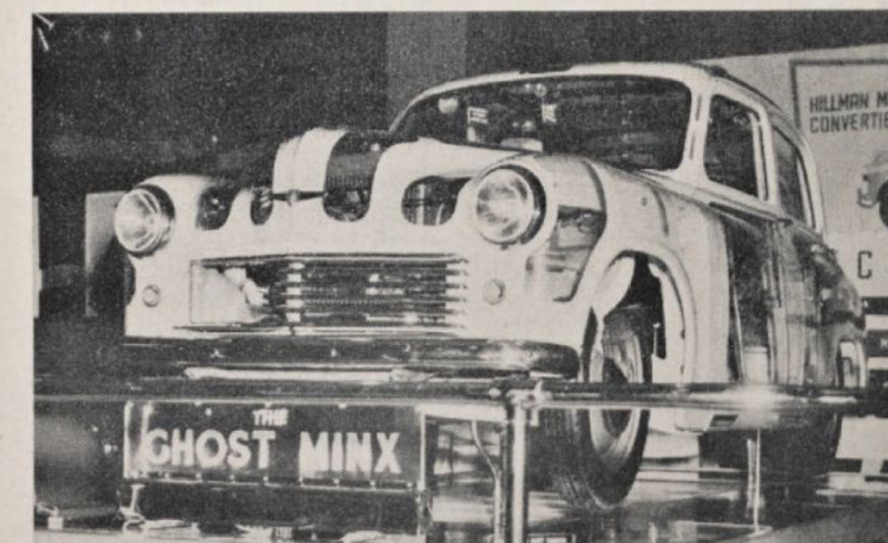
STRIKING eye-catcher was the Hillman Minx ghost car which offered spectators an X-ray eye view of the four door body and chassis
