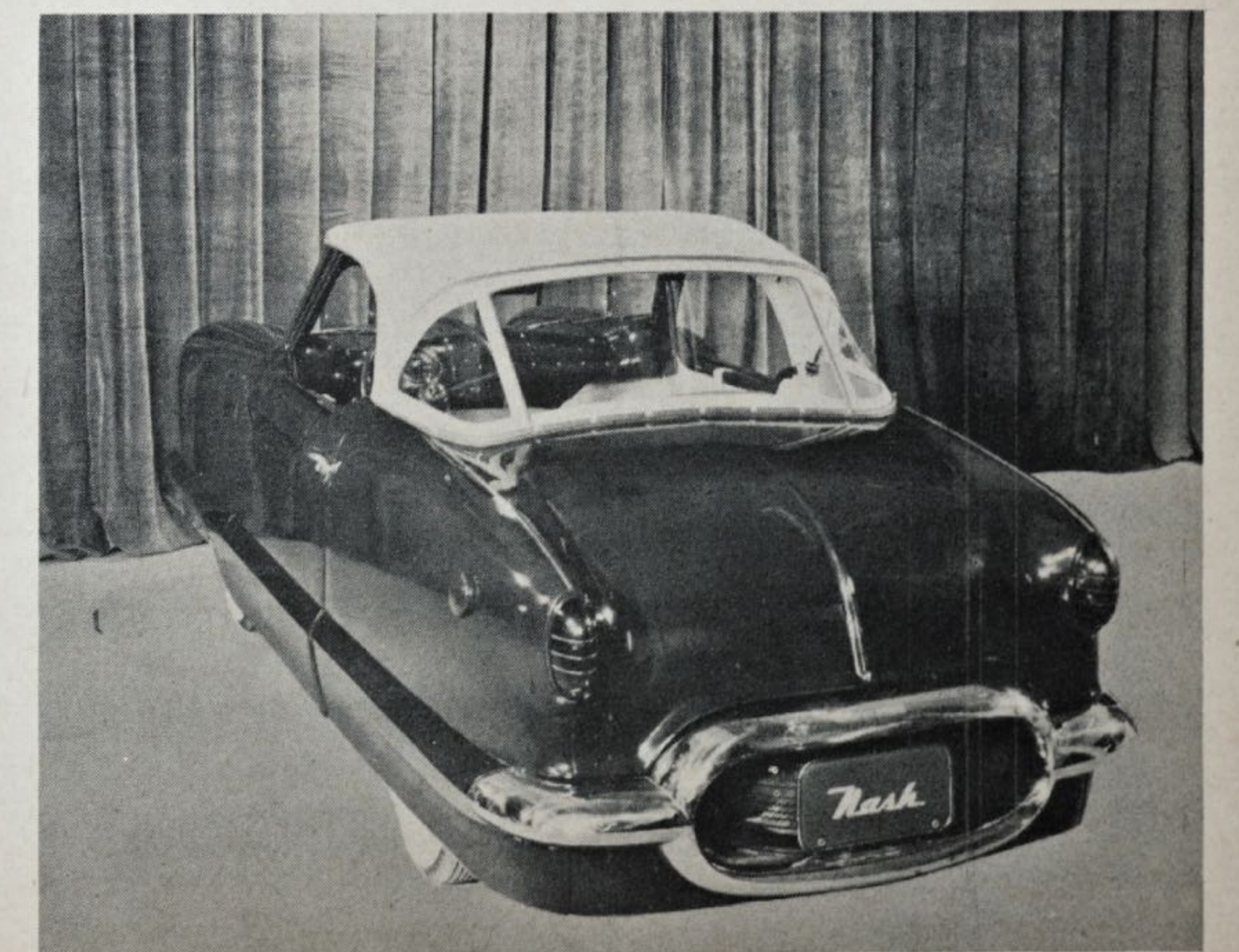
SPARE tire is stowed in a convenient position and is protected by the bumper
