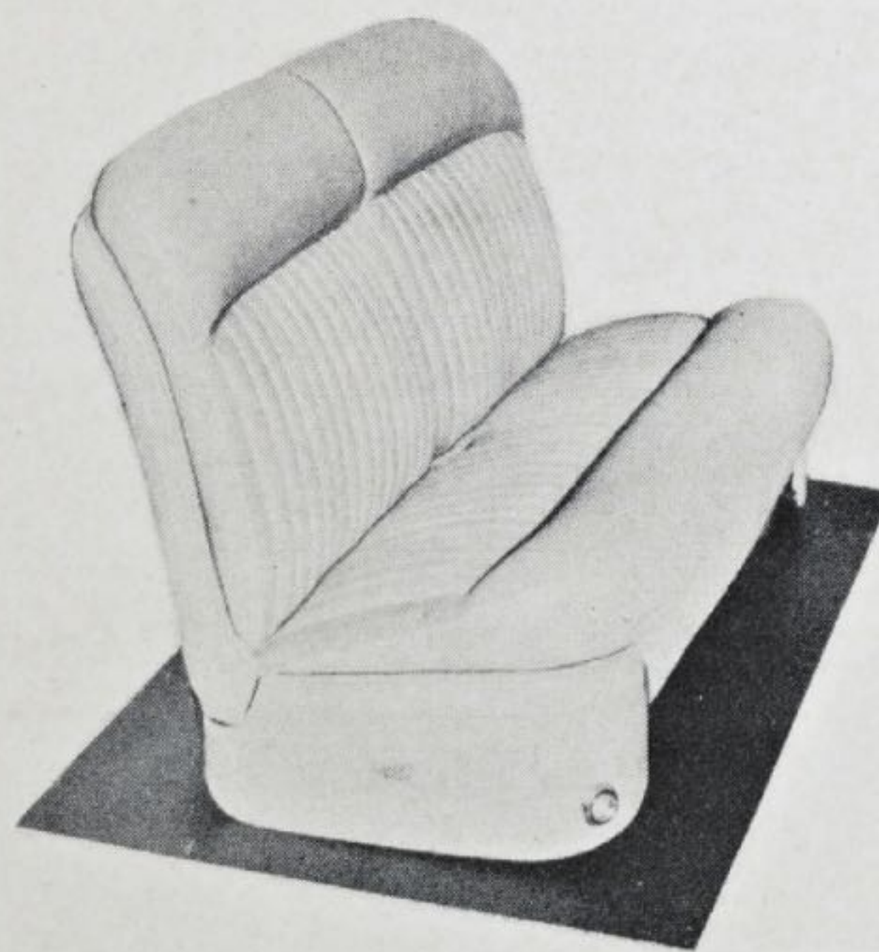
SEAT for Buick, upholstered by Runyan, has airfoam cushions, steerhide covered
