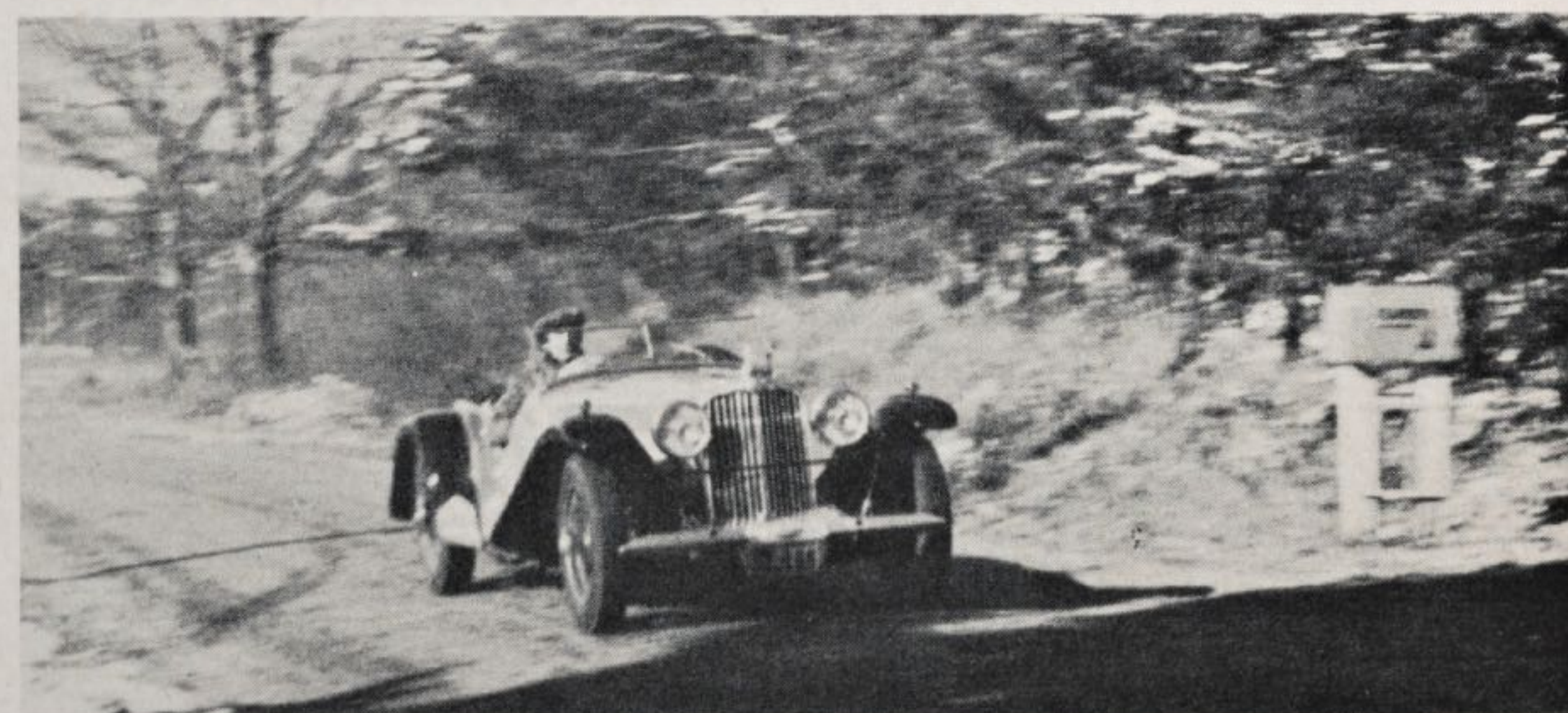
DAVID MITCHELL, Brooklyn, N. Y., is pictured in the hill-climb event in an all-aluminum bodied 1937 model 120 cu. in. A.C. The initials A.C. are derived from the original name of the British company, Auto-Carriers, Inc. The engine is of six cylinder aluminum block design, wet cylinder liners. Power output is about 74 bhp at 4500 rpm
