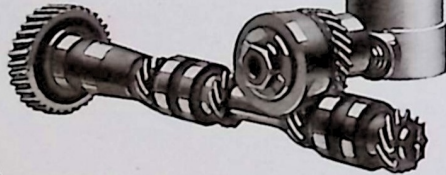
View of Valve Shaft with Sleeve and Cross Shaft of 12 h.p. Argyll Engine
