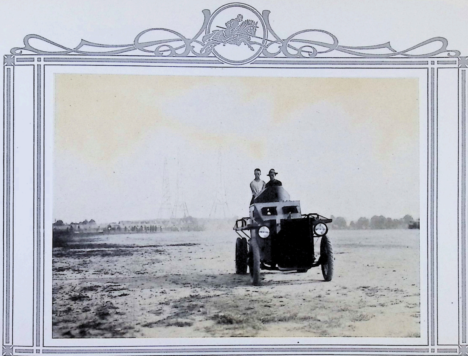
Cross country speed test. Just before attaining maximum speed on first test. Speed here about 40 miles per hour.
