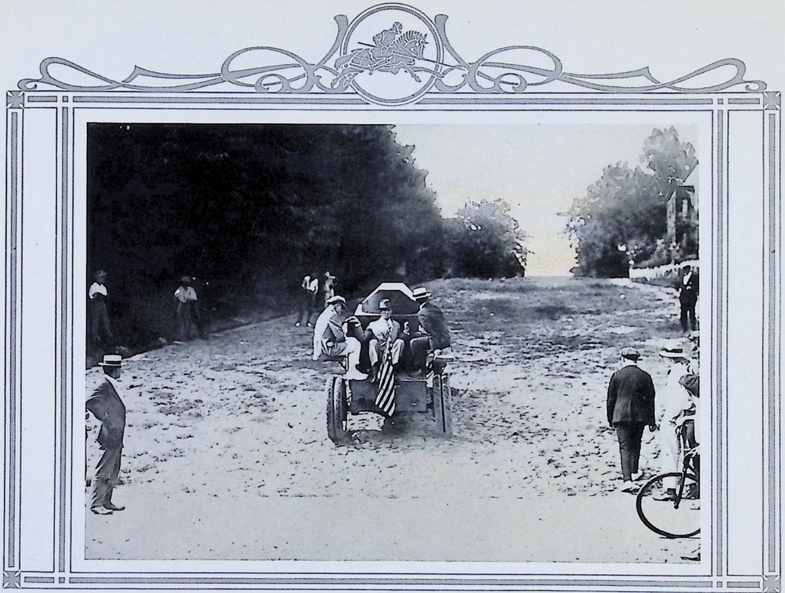
35th Street Hill just after starting climb. Grade, 20% first 18 feet, dropping to 11% remainder of block.
