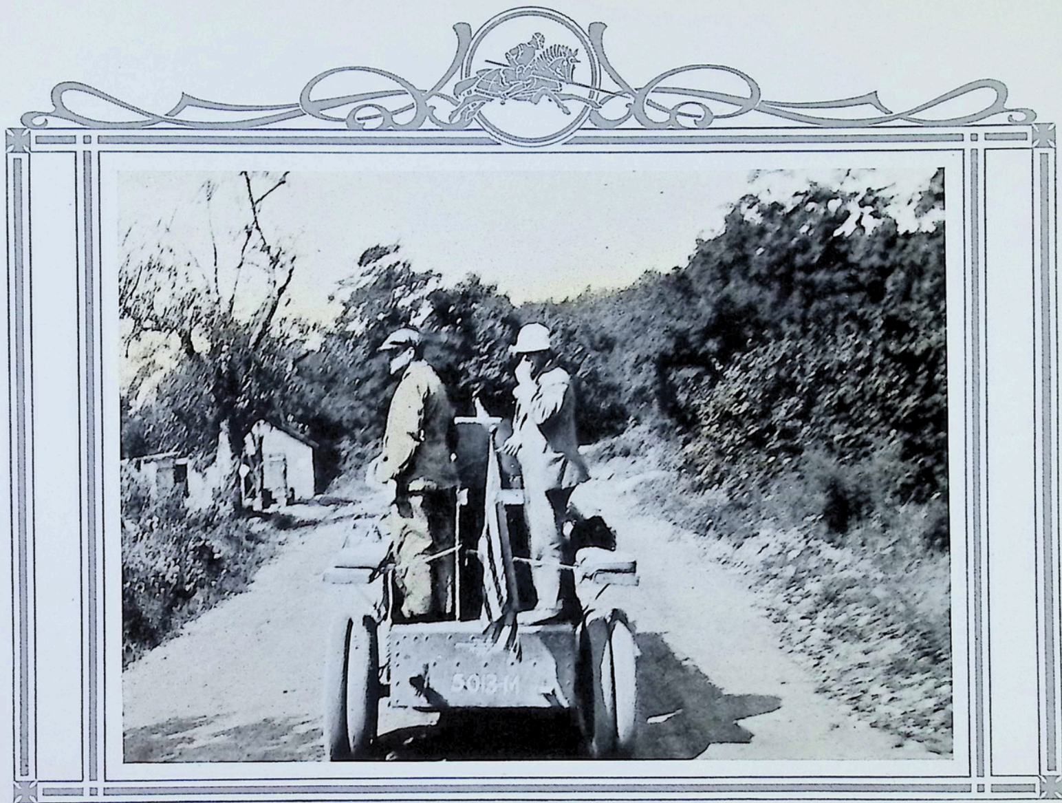
In Allegheny Mountains on New York to Rock Island, Ill., test run. Grade 14%. On second speed, 26 miles per hour.
