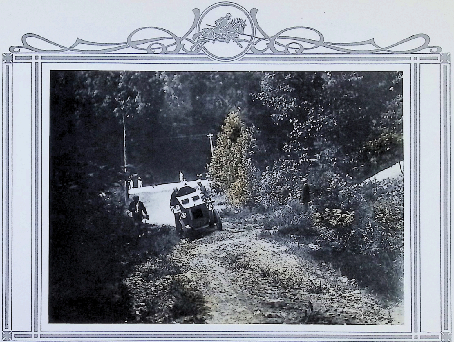
Second trip up hill with Major Casad and Major Ellis aboard. Car negotiated hill on second speed, attaining speed of 20 MPH at summit.
