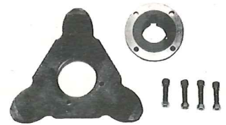
1. Flame hardened drive sprocket connected to drive hub by safety shear bolts to avoid breakage in event of obstructions jamming gutter chain or freeze down. Should this happen drive sprocket is held in place until safety shear bolts are replaced. Drive sprocket is reversible for longer life.
