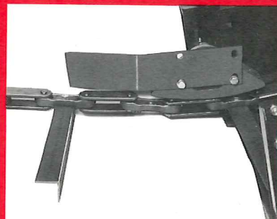
3. Adjustable cast hold down and return shoes at base of elevator guide chain smoothly both up the elevator and into the reverse curve. Hold down and return shoe are interchangeable for longer life.
