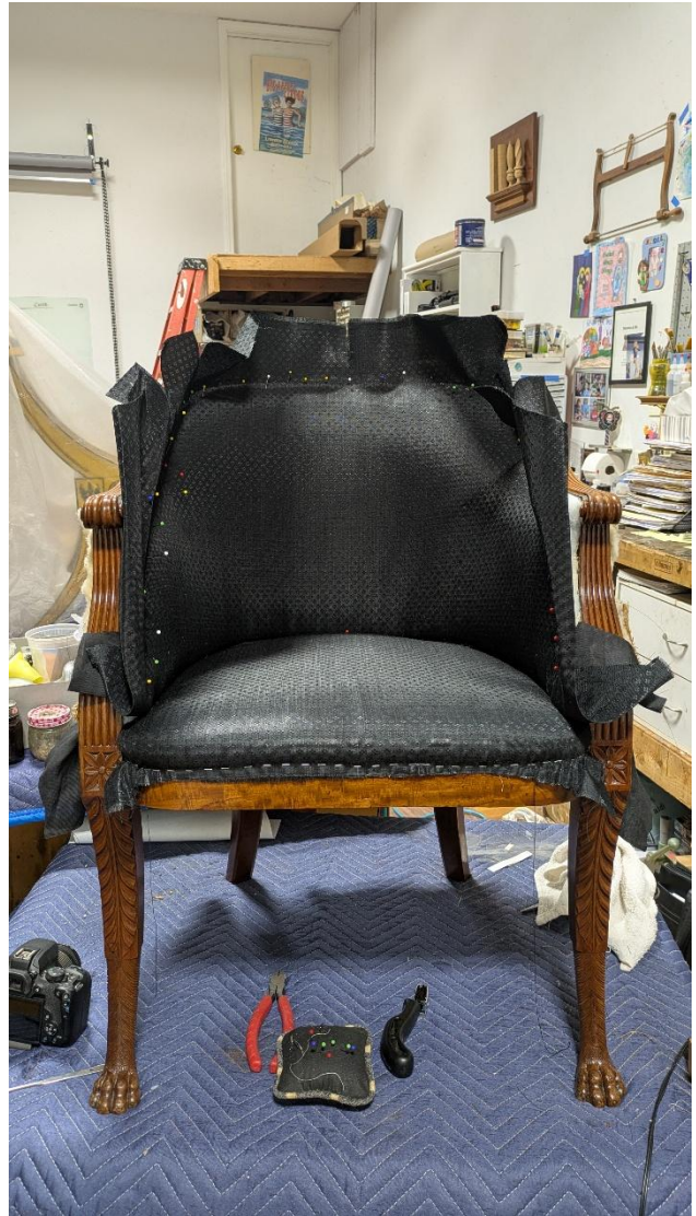
Smoothing out the horsehair of the inner back
