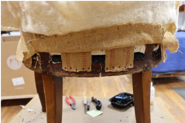
Four pieces of webbing support the burlap for the outback
