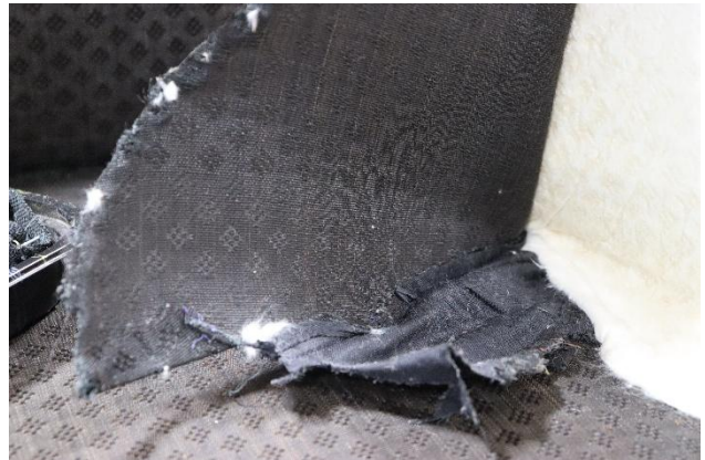
A black cotton pull fabric was sewn to the bottom edge of the inner back show cover
