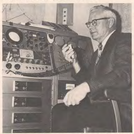
James W. Hill, senior radio technician, sits at maintenance console which keeps constant check on all microwave relay stations. These relay stations allow county-wide communication for Sheriff's Department, County government officials, road maintenance department as well as county-wide emergency networks. Hill is in charge of buying, installing and maintaining all radio and electronic equipment for the County. (San Diego County Photo)
