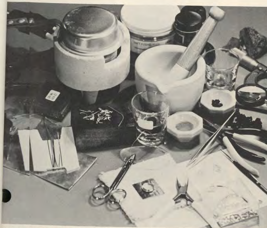
Some of the raw materials and instruments used in the process of creating a jewel; enamel, 3-inch kiln, calipers, gold and silver, preliminary drawing and wire work.
