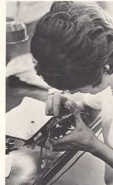
Here, an inspector checks the solder workmanship on an etched circuit board contained in the electronic thermometer.
