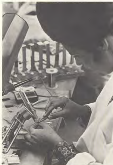
One of IVAC's production employees is pictured here dressing the leads in preparation for making solder connections to the electronic thermometer probe cord.
