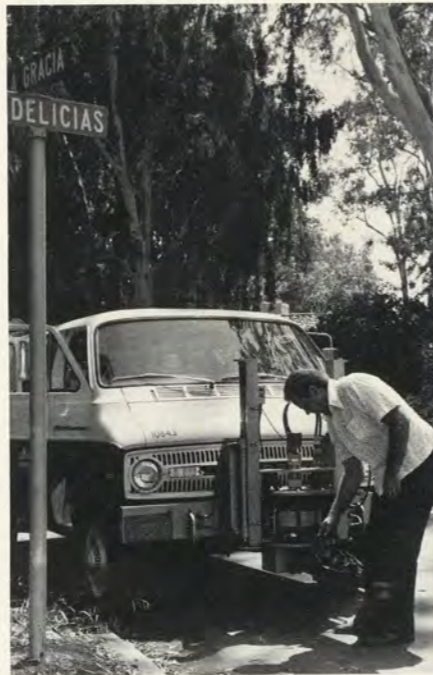
Tony Miller of the Engineering Materials Testing Division of the San Diego County Engineer's Department prepares to test a road in Rancho Santa Fe using the County's new road-rater. The road-rater monitors the condition of a highway and enables the operator to determine if the road needs recapping. The testing division also checks all materials used in the building of County roads to assure a quality product.
