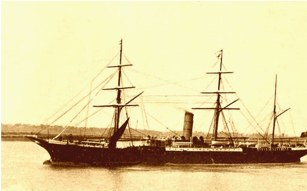
Here we see the S.S. Aorangi as built with a full rigging for sails and a shorter funnel
