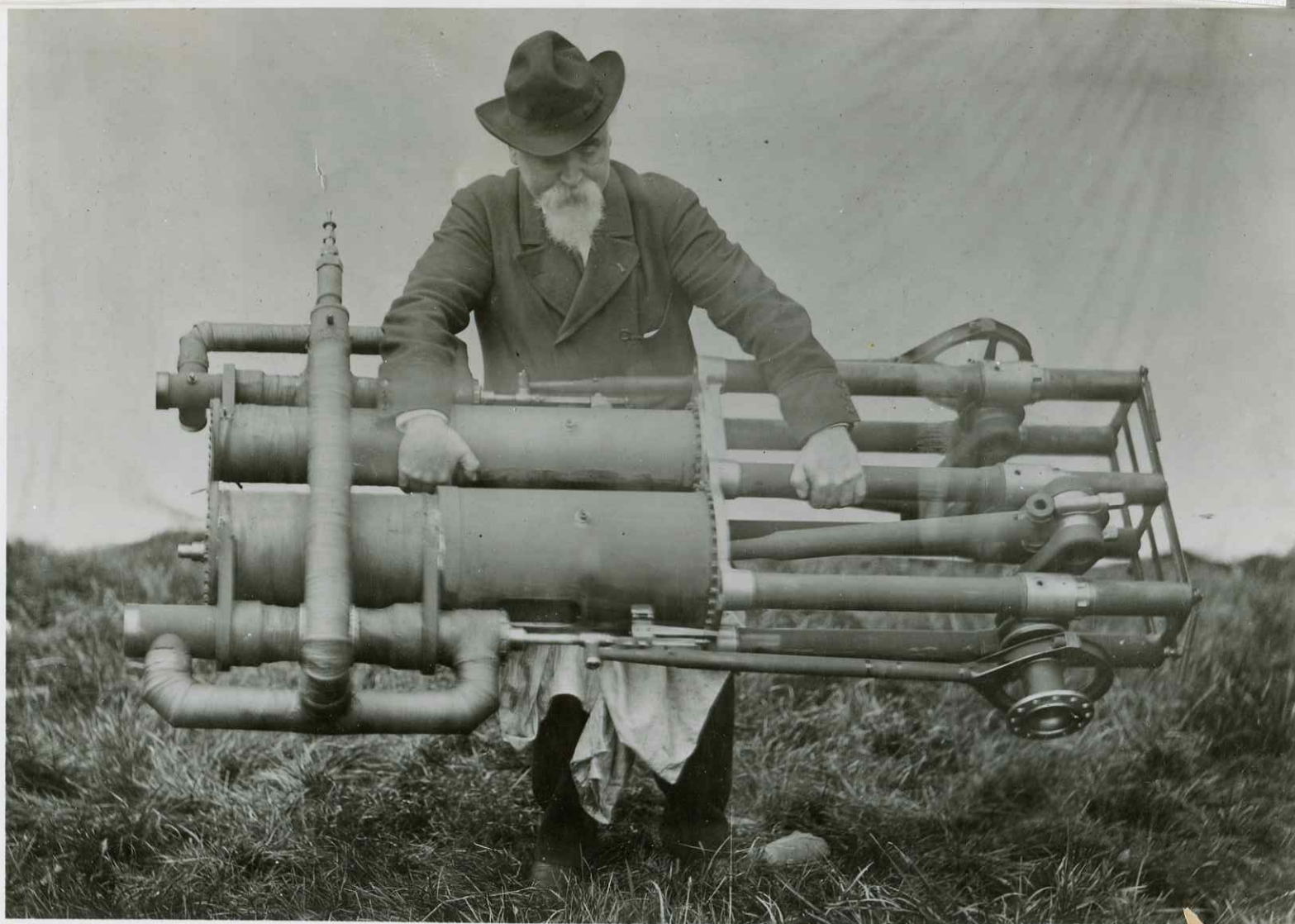
Sir Hiram Stevens Maxim holding on his knees one of the two 150 H.P. engines used in the steam driven airplane of 1890.
