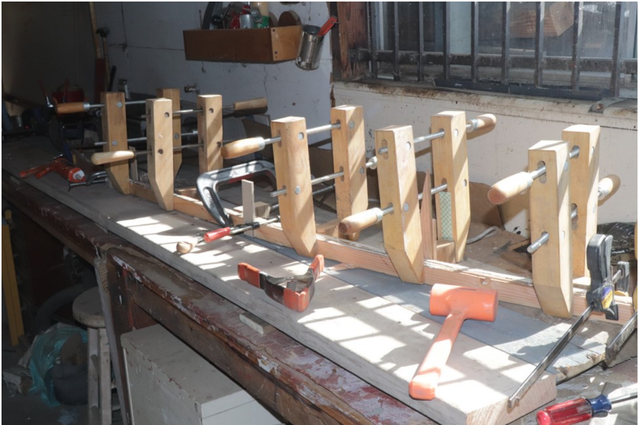
Below - the laminated arch for the Jacumba car #240 platform is slowly taking shape.
