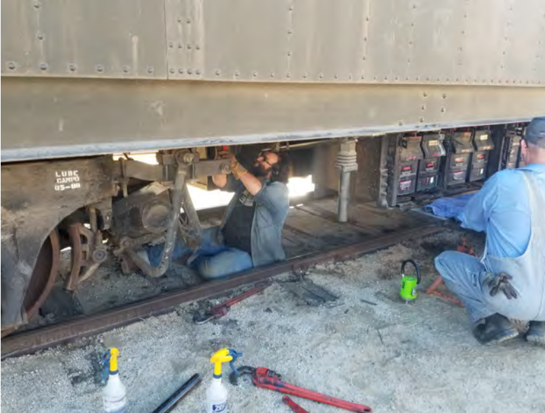
Tim Wamsley is servicing the batteries on ATSF 1509 as Ben Lazerson works to tighten a leaking fitting on the brake pipe.
