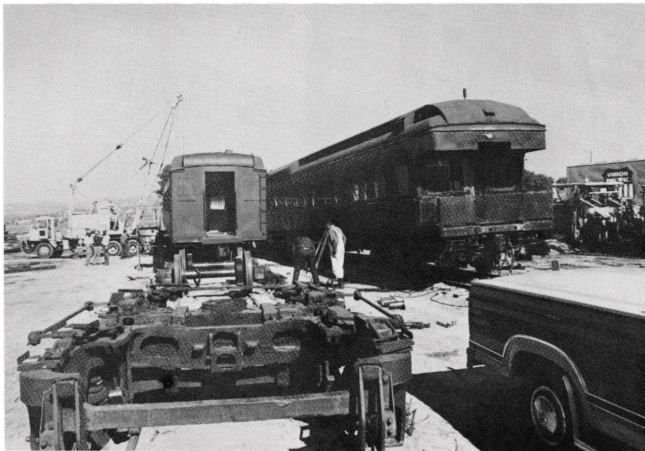
This photo shows the dismantling of the traction motors of our SD&A coaches in full swing. Jim Lundquist and Dan McLean are pulling off axle mounted parts in the center of this scene. Beyond, Doug Mick has the museum crane set up to lift the other end of an ex-self-propelled commuter car so the process can be repeated. At right is our private Pullman ROBERT PEARY , which will soon be used to convey the MTDB board and other officials from San Diego on an inspection of the SD&A all the way to Jacumba. (L. Rose photo)
