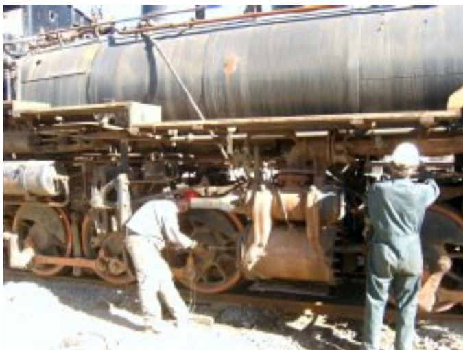
Mike Lucek and Bob Nickles pull the piston into the right high pressure cylinder on #46. Jim Baker photo
