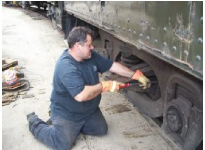
Dave DiGiorgio replacing a brake shoe. Maintenance is one of Dave's many jobs with PSRM.
