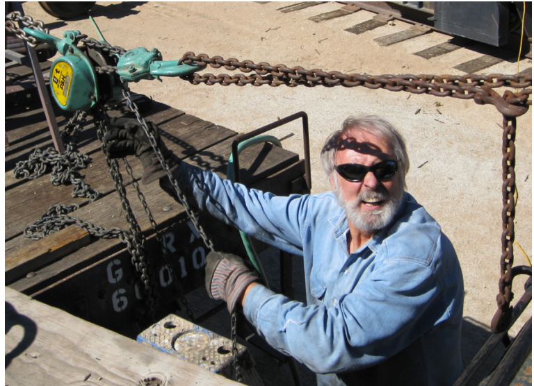
Larry Owen pulls the flue with the chain hoist.
