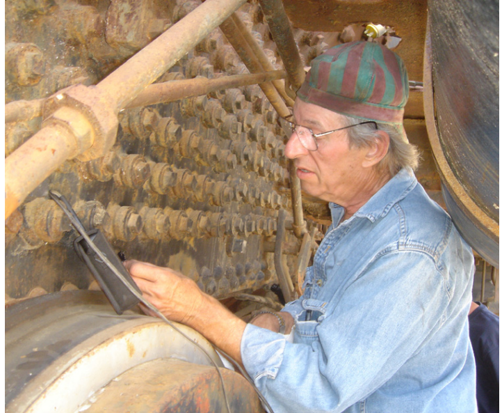
Dave Griner demonstrates UT examination of the Coos Bay #11's boiler.
