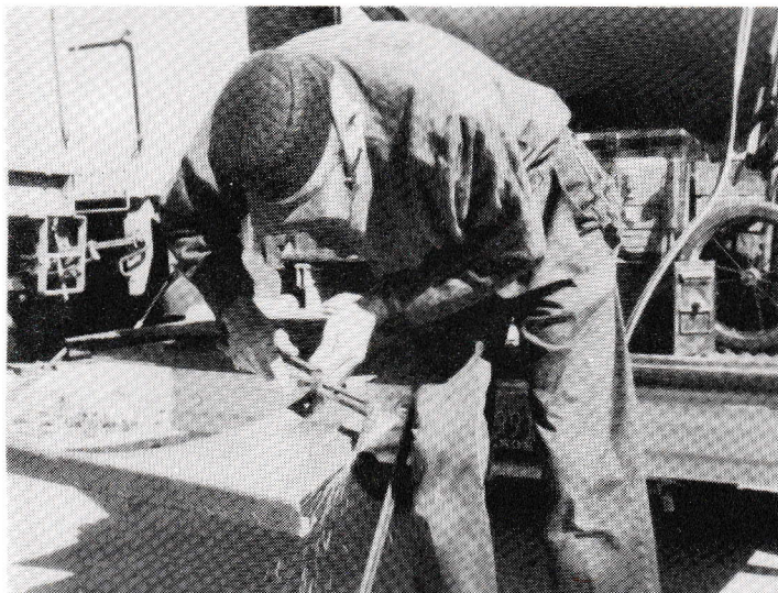
Dick McIntyre cutting a metal patch for the Chief Manajaka.
