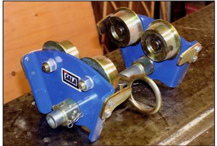
The trolley assembly that runs along the rail prior to installation. There will be two on each rail.
