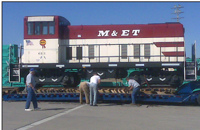
SP 5119 (M&ET 613) being secured to the trailer after loading in Modesto. Ron Hyatt Photo
