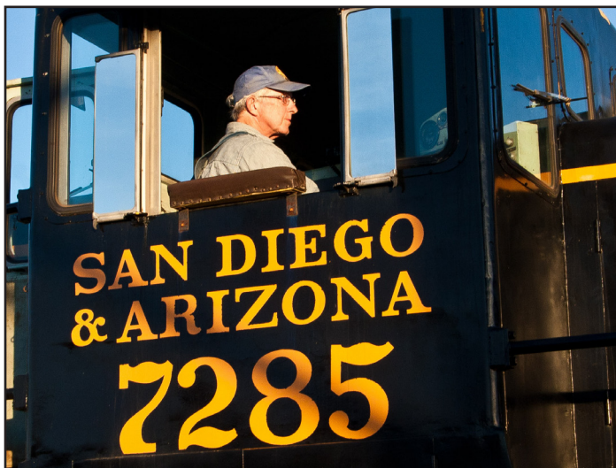
Engineer Rob Stebbins at the controls of SD&A 7285, the museum's 80-ton GE switcher.
