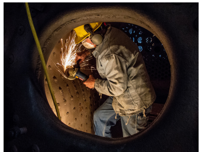
Steam Foreman Jim Baker grinding locations for ultrasound readings in the firebox of Coos Bay No. 11. John Wright Photo
