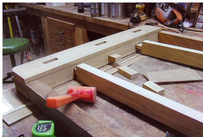
Fresh baggage cart mortises, tenons and stringers. Frank Stites Photo
