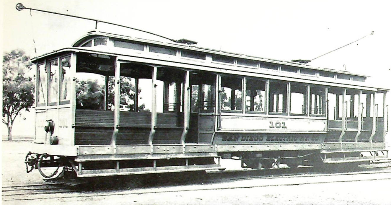
San Diego Electric Rly. Co. No. 101 at Coronado. Car was equipped to pull trailers and did so in Coronado service. It is a wood "California" type car (open-closed-open). Most cars of this type were converted to one man and sides were enclosed. Built by SDER in May 1910. Double truck. 40', 34,100#, 2B-27G, 2GE-202 and K-11 (changed to 2GE-219 and KF), seats 44. (Southwest Rly. Library - R.V. Dodge collection).
