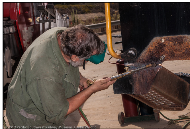
Rusty Hoar torches the steps off the rear of 3709 to provide clearance for the trailer. John Wright
