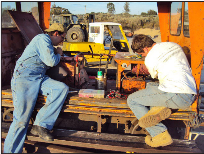
Hector (Left) looks at the rotating beacon and headlight wires while James (Right) repairs wiring to the horn.
