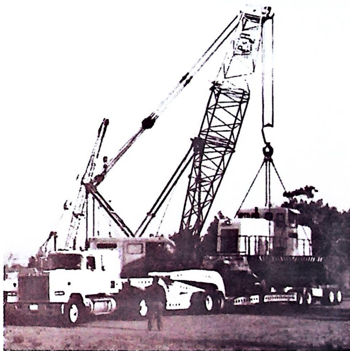
Massive donation of time and effort is evident as our 80-tonner is lifted off a Marine Corps transporter by a USMC 80-ton crane at Stuart Mesa. Photo by B. Schneider
