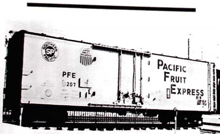
Ladders, brakewheel, rooftop walkway, and sliding plug door with hinged extension show in this January 1993 view of PFE #11207 near the La Mesa Depot.
