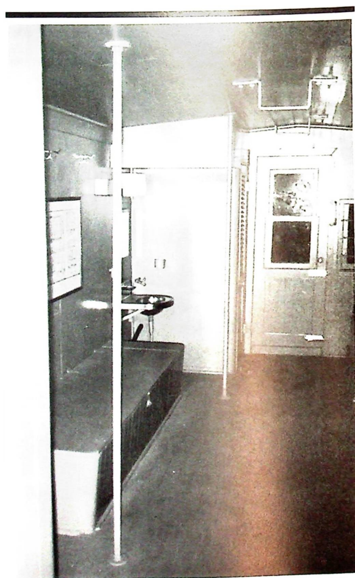
Beautifully restored interior of SP #1058 shows its steel sink, brass coathooks, toolbox/bench, door windowframes, overhead stretcher holder, and restroom. Photo B. Schneider
