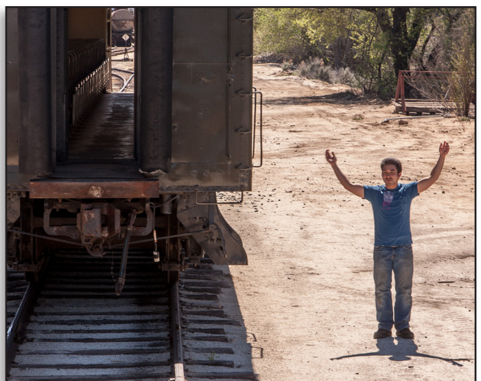
Brakeman Trainee Raymond Lee gives hand signals to the engineer in preparation for coupling up.
