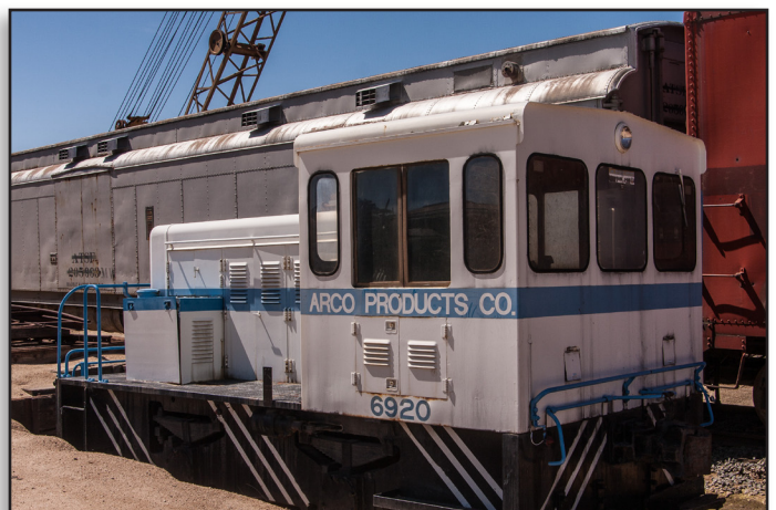
Arco Products 6920, built by Balwin-Lima-Hamilton, is the museum's only diesel-hydraulic switcher.
