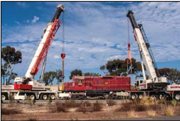
SP 3709 in the process of being lifted off its wheels prior to being transported to Campo. John Wright
