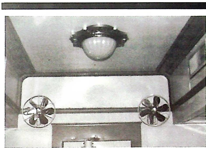
The brass light fixtures and fans in ATSF #1509 never shone more brightly than they do now! The light globes in the newly-restored care are also new - in the 1940's style.
