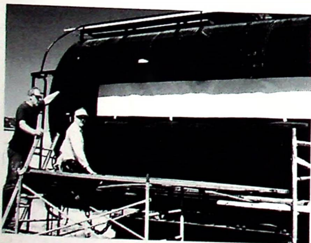
Larry Owen and James Balnis position the stencil and apply the paint placing the familiar Southern Pacific block lettering on the tender.
