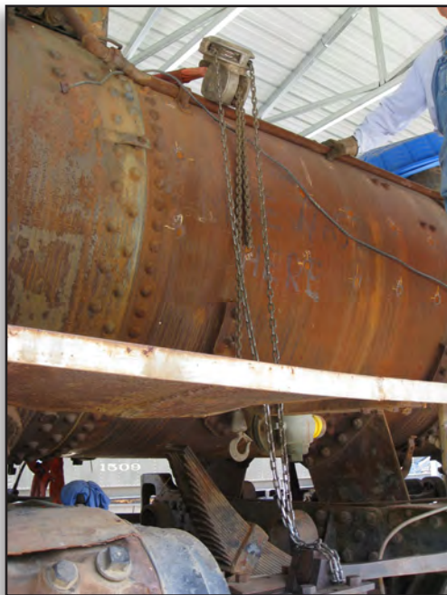
Chain hoist set up to lower springs to the ground.
