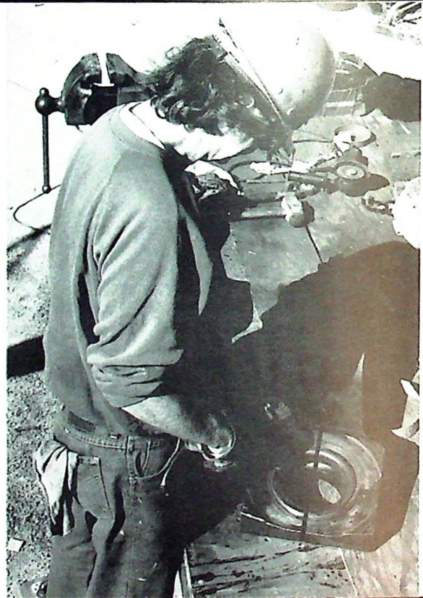
Bob Nickles, Steam Team member and Museum locomotive engineer, burnishes 2353's valve motion eccentric crank prior to installation of the driver pin on Nov. 11, 1995.
