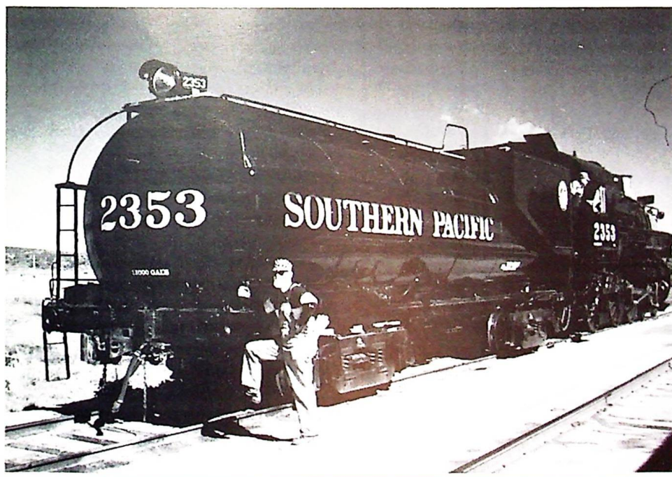
Brakeman/Training Officer/Steam Team member Jim Baker awaits the next move at the rear of Vanderbilt 120-C-1 tender SP #8540. It is lettered in post-1946 style, with "Lines" deleted from its sides and the number on the rear enlarged from the earlier smaller size. Light and loaded tender weights are on the sides of the water tank beneath the oil tank, with new SDRM emblems above. Built in 1922, she's beautiful and so modest she doesn't even display her own number!
