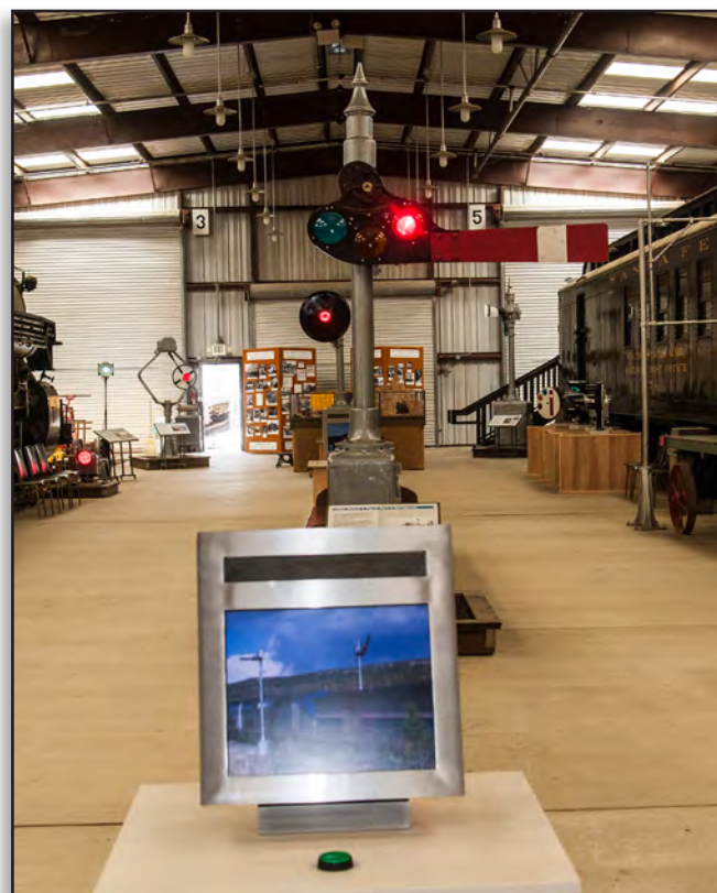
Union Switch & Signal Style S semaphore showing a stop indication. In the foreground is the interactive display. John Wright
