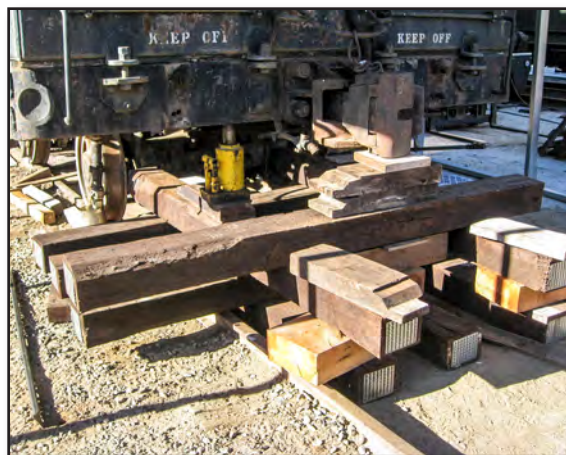
The cribbing and jacks used to raise the rear end of the engine. Jim Baker
